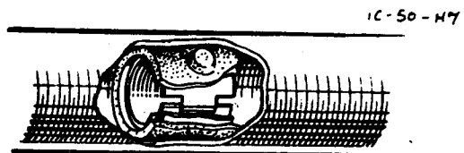
Fig. 5. CUTAWAY VIEW OF AN OUTER COLUMN BUSH
